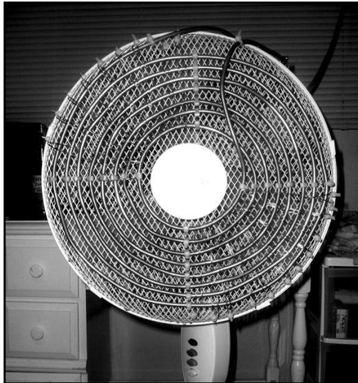
**Figure 1: Fan With Attached Copper Coil**
